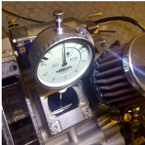
Figure 5-5 – Dial Indicator Lined Up and Calibrated to Zero, Ready for Measurement.
