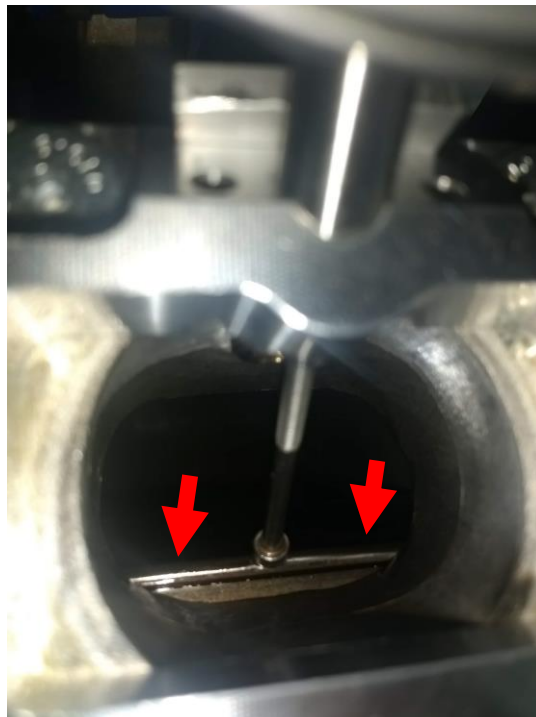
Figure 5-6 – Push Down in the Direction Indicated Until the Spring is Fully Bottomed Out.
